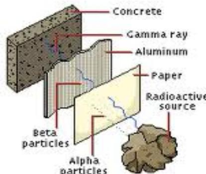
Fig.1.Radiation penetration (source <http://www.xenu.net/archive:>
