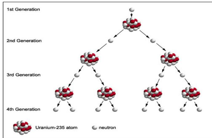
Fig.3. (b) Chain reaction (source: [www.atomicarchive.com/fission/fission1.shtml](http://www.atomicarchive.com/fission/fission1.shtml))
