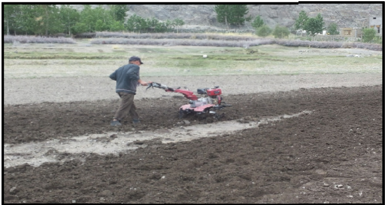
Fig. c. Power tiller being used for ploughing field in Nubra in 2016.
