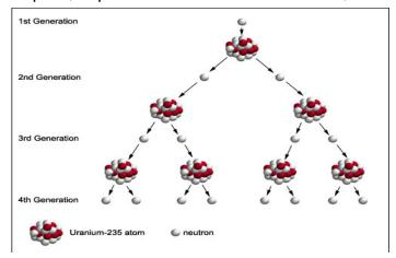
Fig.3. (b) Chain reaction (source: www.atomic archive.com/fission/fission1.shtml)
