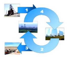
The nuclear fuel cycle begins when uranium mined, enriched, and manufactured into nuclear fuel, (1) which is delivered to a <u>nuclear power plant</u>. After usage in the power plant, the spent fuel is delivered to a reprocessing plant (2) or to a final (3) for geological disposition. In <u>reprocessing</u> 95% of spent fuel can potentially be recycled to be returned to usage in a power plant (4).
